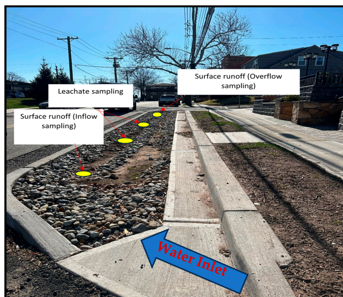
Figure 1. Lysimeters locations for sample collection and inlet flow direction. (Image credit: authors).
